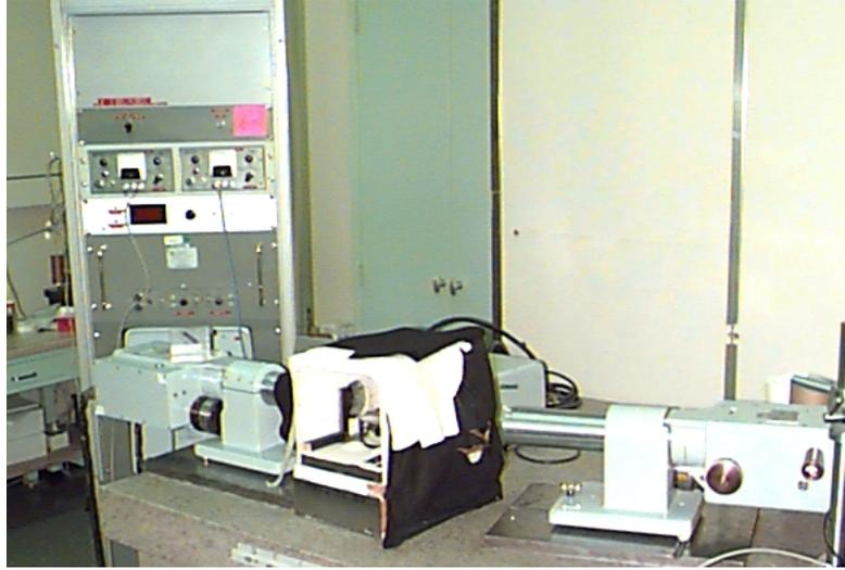
The central box holds a serrated anvil with two brass positioning pins glued to the surface. The ends of these pins are the reference points for positioning the angle blocks. The box has a cloth cover that should be closed during the measurement to prevent air currents that make the autocollimator output noisy.
